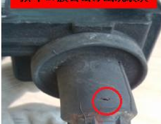
损坏 2: 胶套击穿出现裂纹
